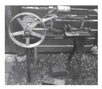
A mechanical engineer, who collected old tools and was moving out of state, donated our saw. The saw had been left out in his back yard for several years, and the rain had rusted and frozen many of the moving parts. Most of the parts were intact, however, with the exception of some connecting rods and a broken wing nut (more on that later).
